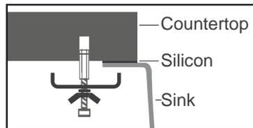
POSITIVE, when the sink is protruding above the
