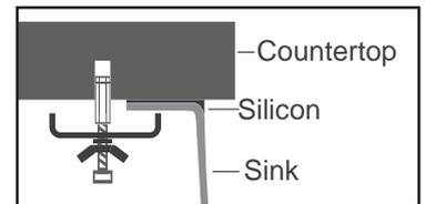
NEGATIVE, when the sink is installed in the niche of the countertop.
